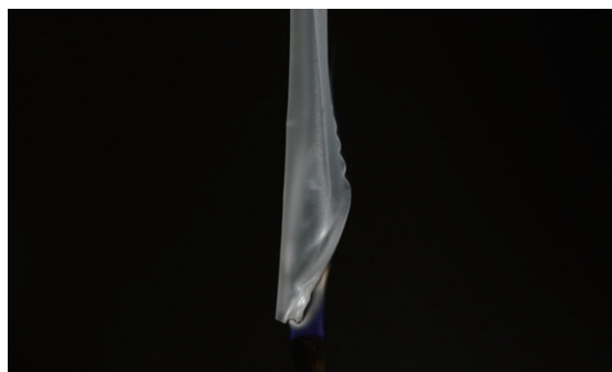
6% loading to PP (100µm VTM-0)
